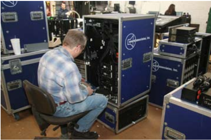
ABOVE: Brother John Gibson carefully wiring an equipment rack in preparation for installation on "Enron."
